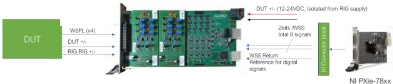
The unit is designed to used together with FPGA code implemented in LabVIEW FPGA for pattern generation.
